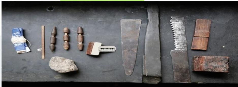
A few of the more than 50 tools used by specialists to make the muslin weaver's *shana* (ultrafine-toothed reed comb) from a dense bamboo called *mahal* that allows for the setting of more than 1,000 teeth per meter. On a loom, shanas keep separation among spiderweb-thin warp threads.
