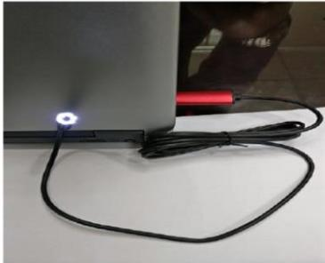
A flexible borescope includes a bundle of optical fibers which divide the image into pixels. It is also known as a **fiberscope** and can be used to access cavities which are around a bend, such as a combustion chamber or "burner can", in order to view the condition of the compressed air inlets, **turbine** blades and seals without disassembling the engine
