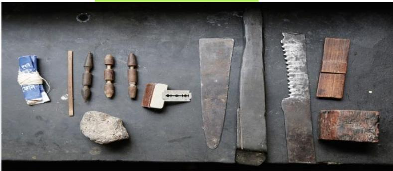
A few of the more than 50 tools used by specialists to make the muslin weaver's *shana* (ultrafine-toothed reed comb) from a dense bamboo called *mahal* that allows for the setting of more than 1,000 teeth per meter. On a loom, shanas keep separation among spiderweb-thin warp threads.
